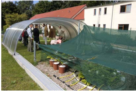
Open field laboratory to simulate water stress draughts on European beech trees
