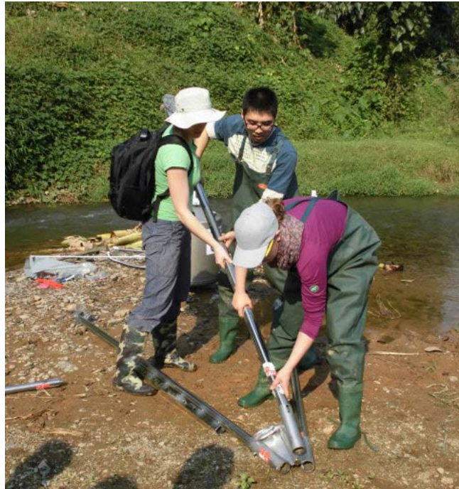
Pic. 10 - Setting up of Freeze-Core
