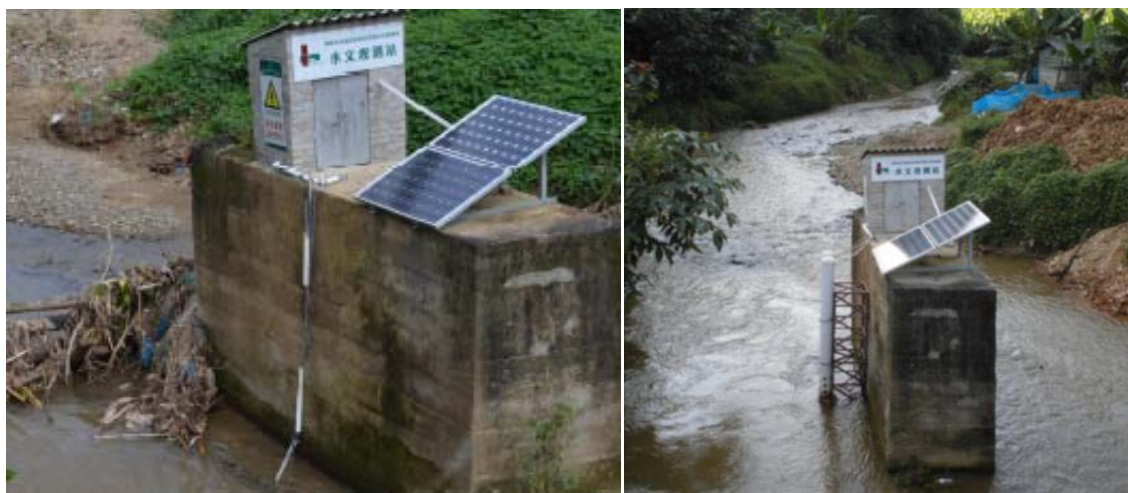
Pic. 9 - Destroyed Monitoring Station P4 after flood (left) and functional Monitoring Station P4 (right)
