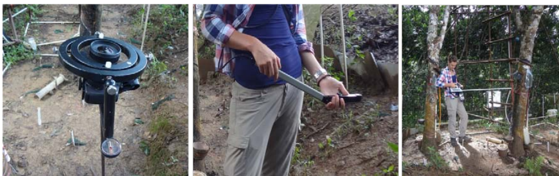
Pic. 1 - 3 - Hemispherical photography method HemiView Delta-T Devices Ltd, Cambridge, UK (left); Gap fraction method LAI2000 LI-COR, Nebraska USA (middle); Light absorption method SunScan Delta-T Devices Ltd, Cambridge, UK (right)
