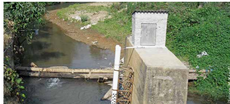
Station for measuring water quality on the Naban River in the Naban River Watershed National Nature Reserve (NRWNNR).
