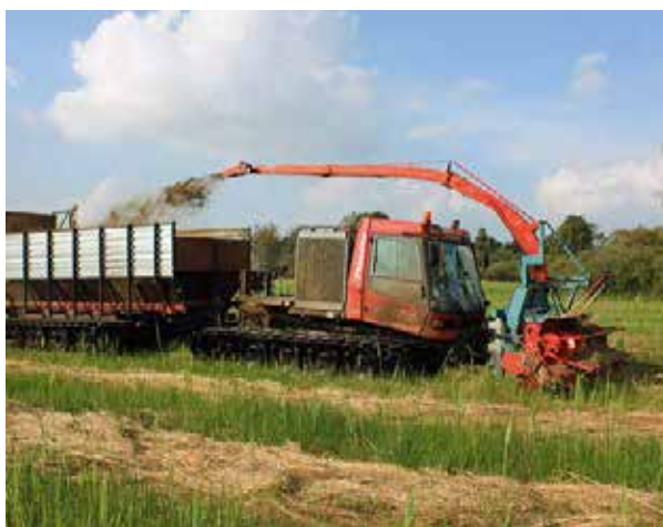
Fig. 75: Harvesting biomass with adapted harvesting machines (Source: C. Schröder).
